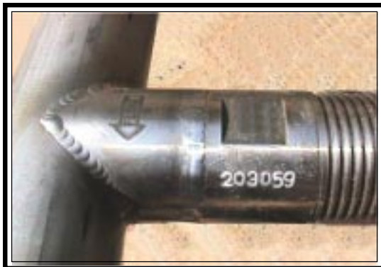
Flow Element Serial Number Also Showing Flow Arrow (Located near the FE enclosure. It is also on the enclosure tag.)
